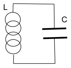
**Example 6**: A capacitor with C = 4.6nF is connected to an inductance with L = 3.2 mH. **a**) Show that the charge (and thus the current) in the cicuit exhibits oscillatory time dependence. **b**) Determine the period of oscillation. **c**) If the capacitor is fully charged at time t = 0 with  $Q_0 = 1.3$  pC, find the maximum value of the current in the circuit.
